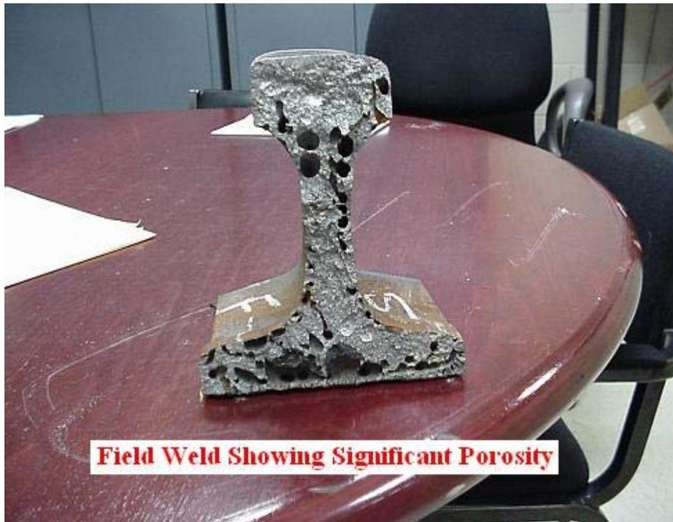
Figure 38: Thermite Weld Showing Severe Porosity
