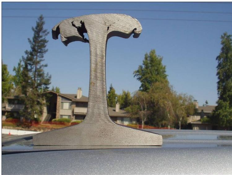
Figure 26: Vertical Split Head (Shear Break)
