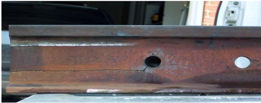
Figure 43: Bolt Hole Crack Originating in Lower Quadrant with Significant Progression
