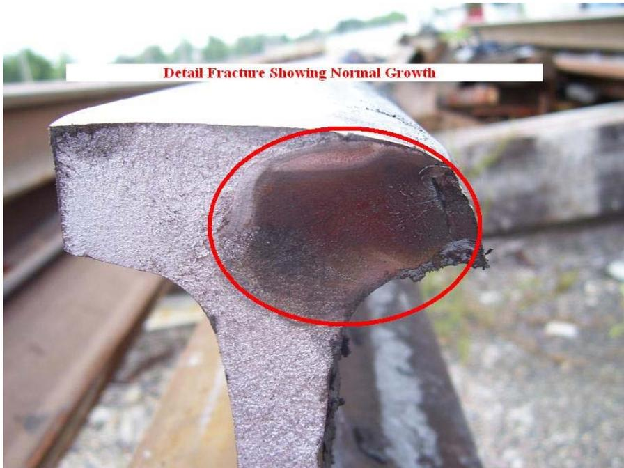
Figure 4: Detail Fracture Showing Normal Growth Pattern
