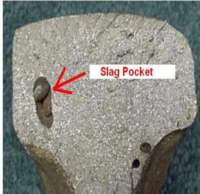
Figure 37: Thermite Weld with Slag Entrapment
