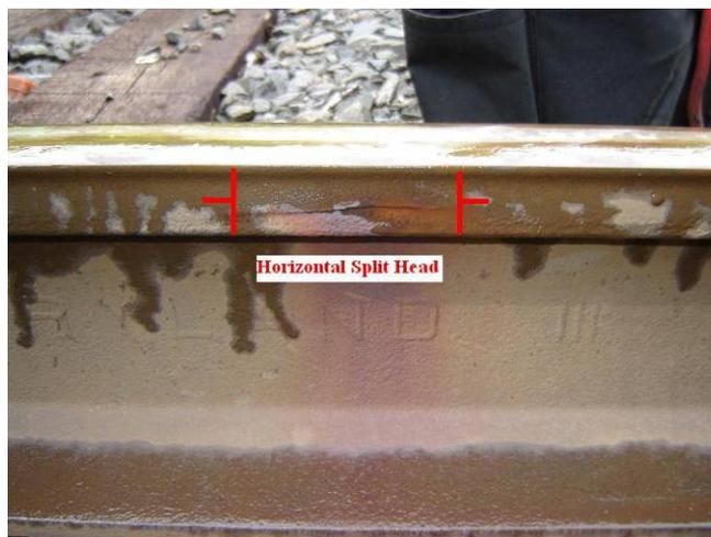
Figure 23: Side View of Horizontal Split Head
