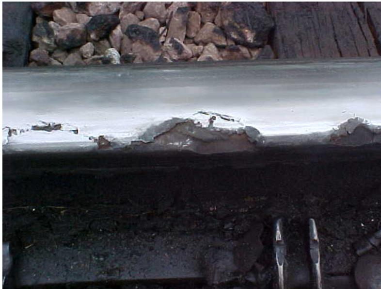
Figure 47: Gauge Side Shell Showing Severe Parent Metal Decay
