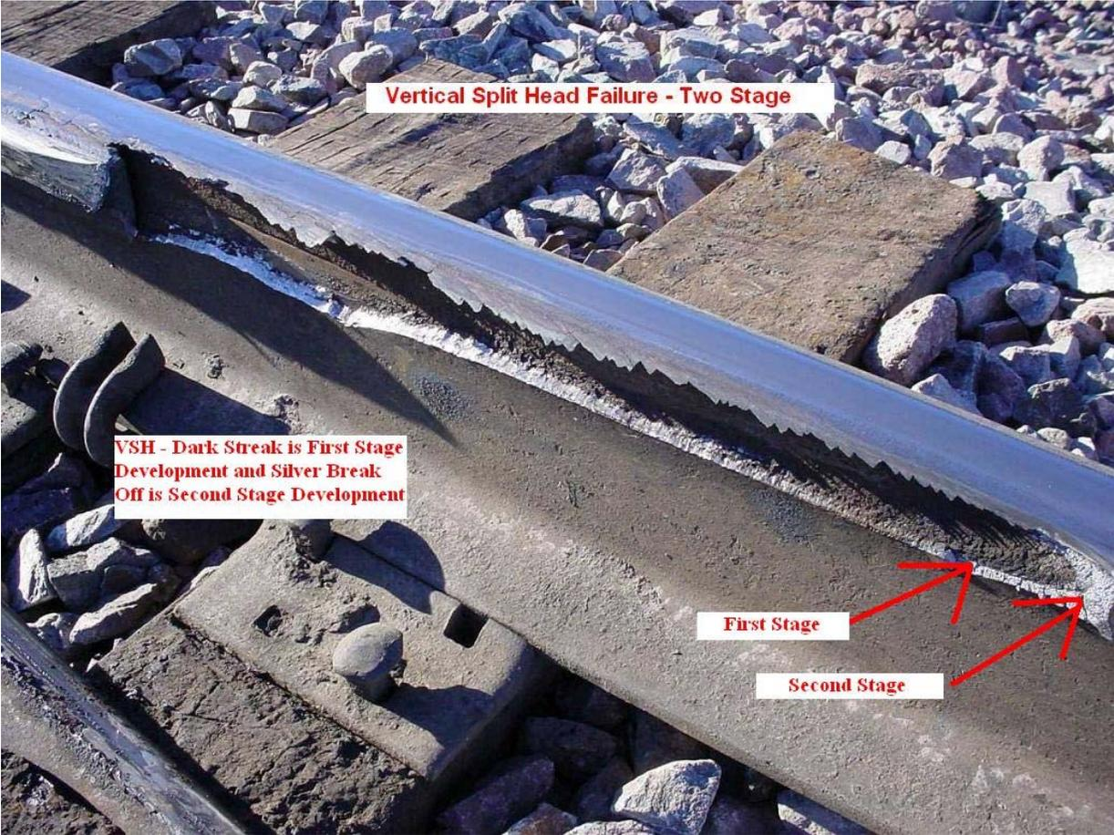
Figure 8: Vertical Split Head Showing Two-Stage Development
