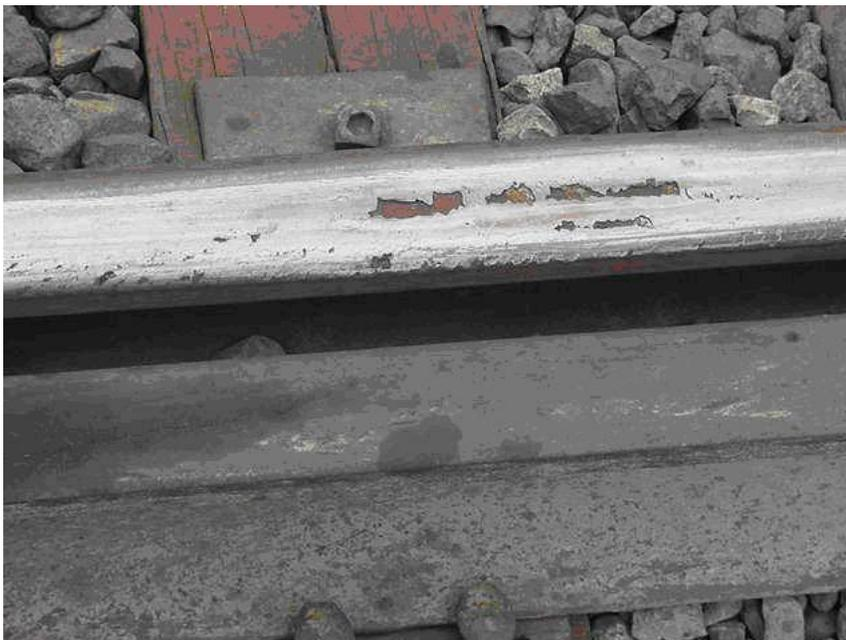
Figure 51: Flattened Rail Head Showing Displacement of Parent Metal (Spalling)
