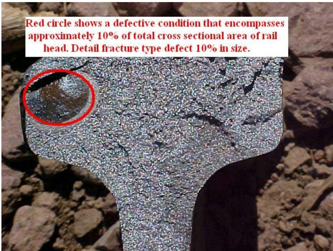
Figure 1: Identifying Transverse Defects in Relation to Cross-Sectional Area of Rail Head
