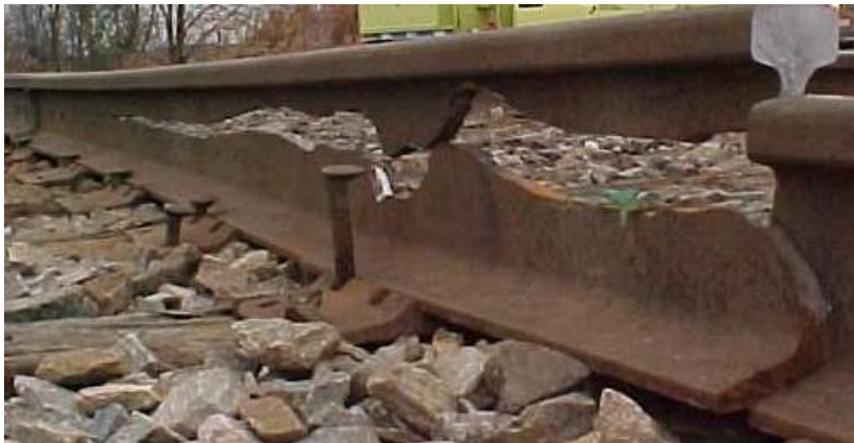
Figure 31: Web Failure Resulting from High Residual Stress
