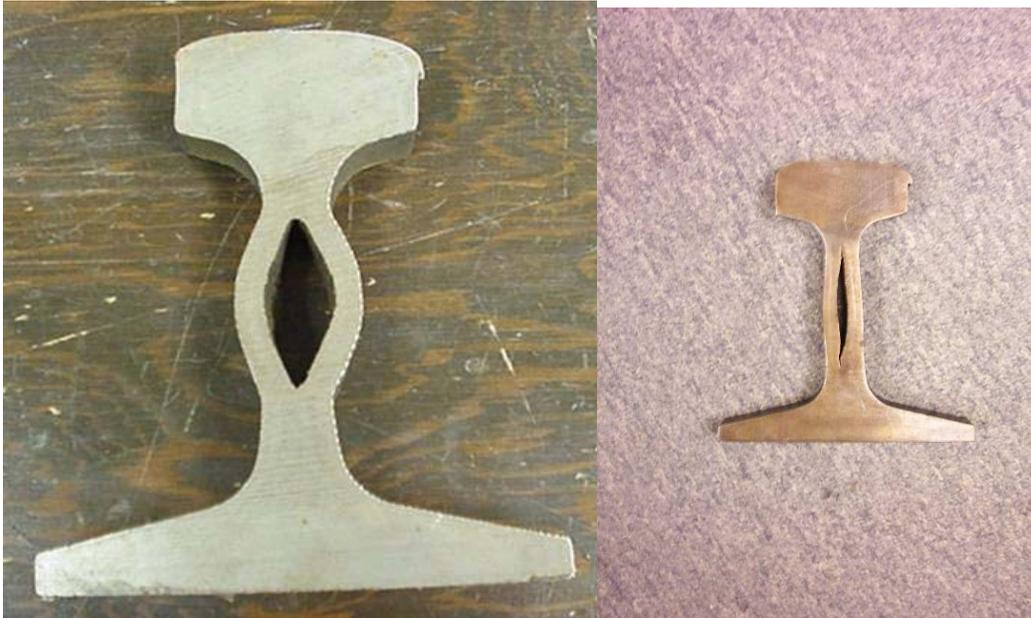
Figure 32: Piped Rail Showing Significant Rail Collapse
