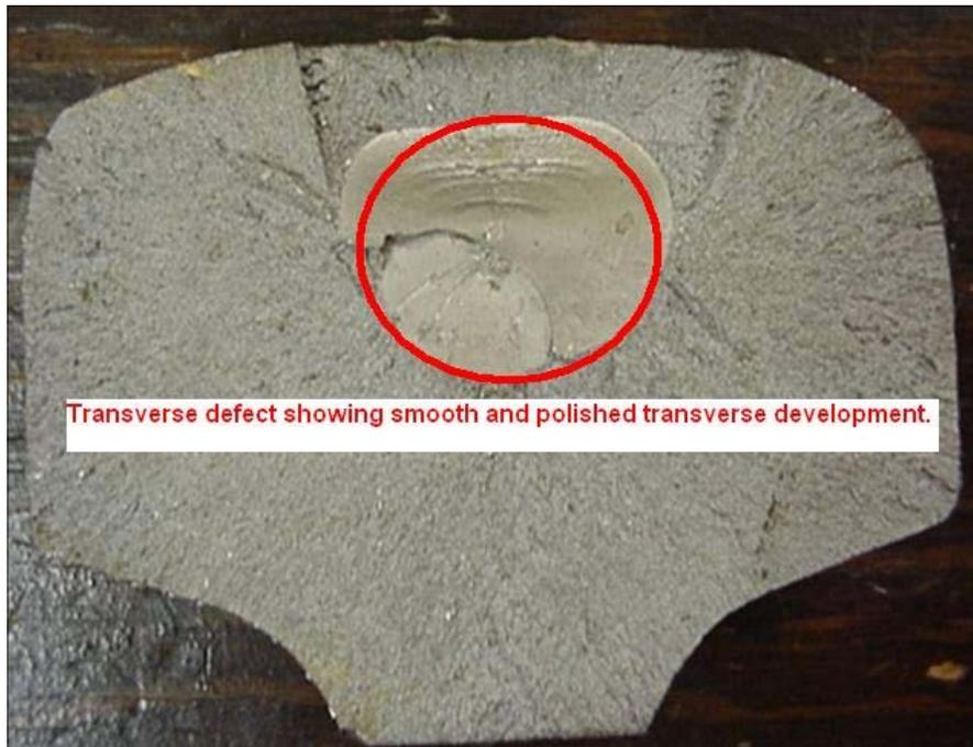
Figure 3: Transverse Fissure Showing Normal Growth Pattern.
