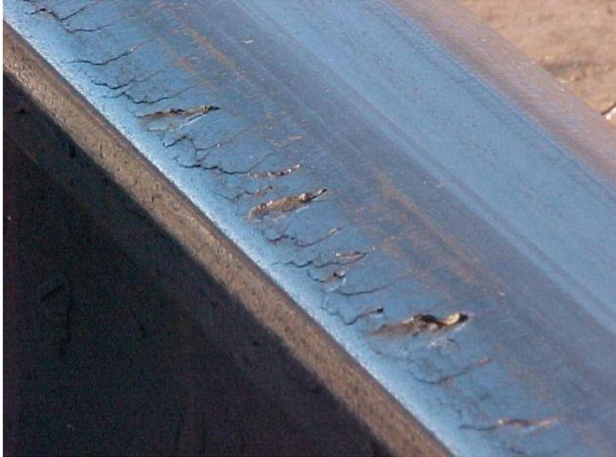
Figure 50: Gauge Side Head Checking and Flaking
