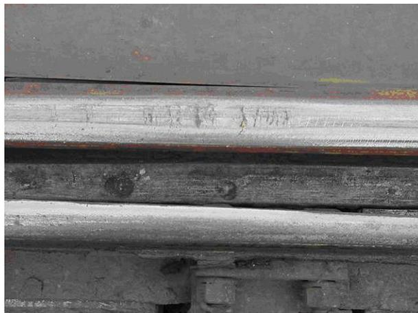
Figure 49: Thermal Cracks on Burned Stock Rail
