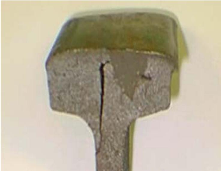
Figure 24: Vertical Split Head Defect Breaking Out in Head/Web Fillet Area
