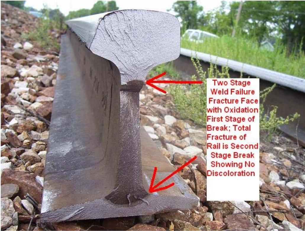
Figure 9: Weld Failure Showing First Stage Fatigue Development and Second Stage Rupture
