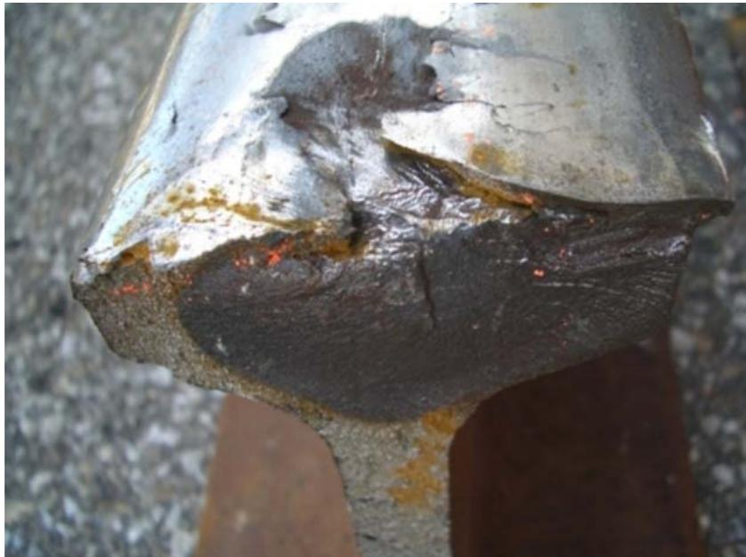
Figure 20: Engine Burn Fracture Showing Significant Growth
