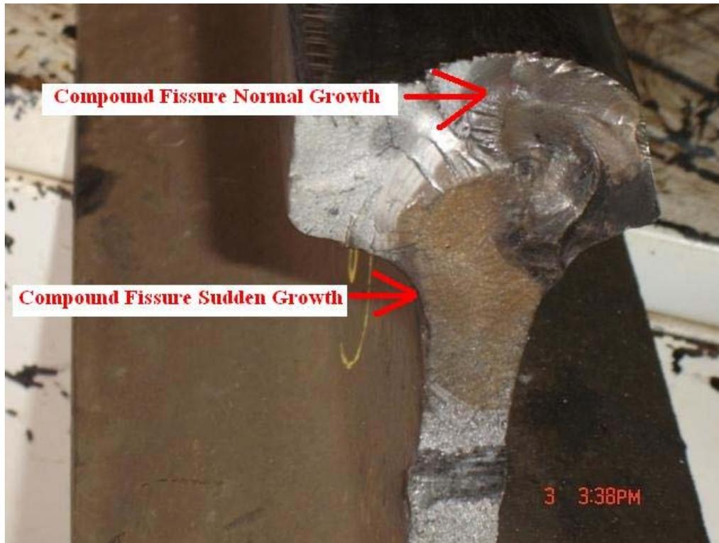
Figure 14: Compound Fissure
