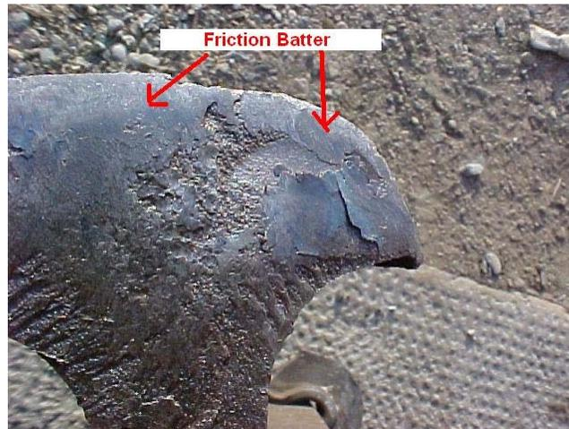
Figure 12: Friction Batter from Fracture Face Contact
