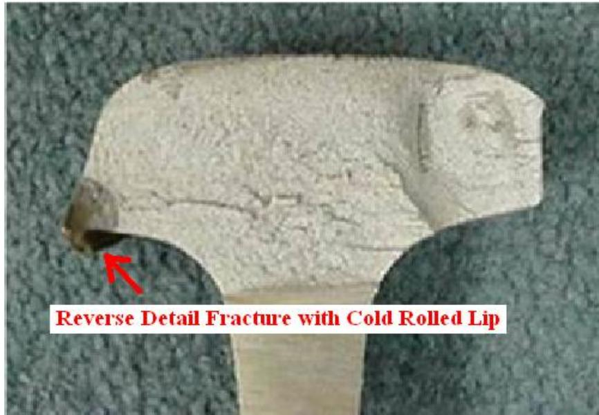
Figure 18: Reverse Detail Fracture
