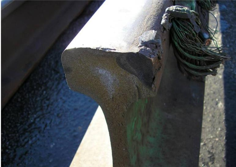
Figure 41: Gas Pressure Weld Showing Oxide Inclusion and Improper Fusion
